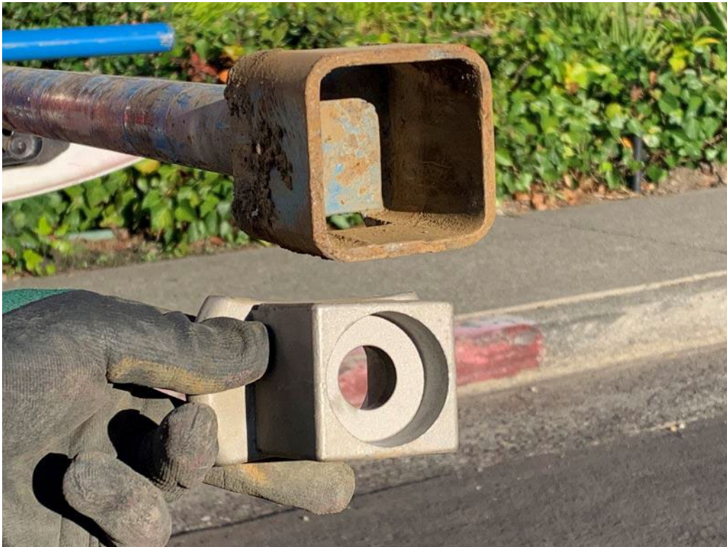
Valve Key With New Operating Nut
